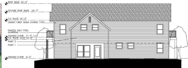
03 North Elevation Bldg 1 (between bldgs) Scale: 1/8" = 1'-0"
